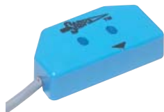
Type E / P1 Sabre Switch (2) SPDT Proximity 1 amp @ 120 VAC, 1 amp @ 24 VDC, 25 Watt Max. Minimum 1 mA
